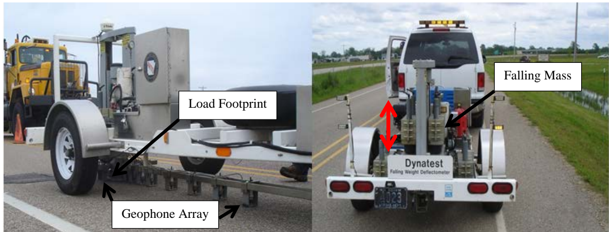
Figure 5.1. Side and rear view of AHTD's FWD at Marked Tree site.
