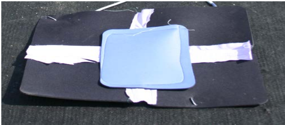
Figure 3.14. Geotextile strain gage protection, neoprene pad (Howard 2006).
