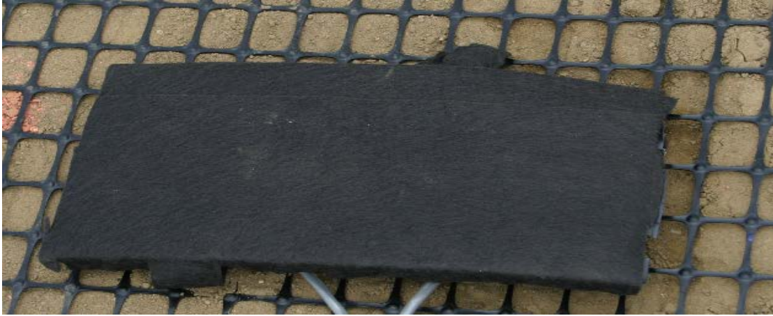
Figure 3.13. Geogrid strain gage protection, strip drain (Howard 2006).
